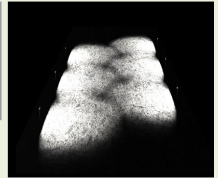
Offset lighting to avoid black spots – accident free driving
